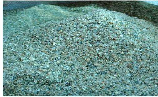
**Gambar Sampel agregat halus (pasir)**
