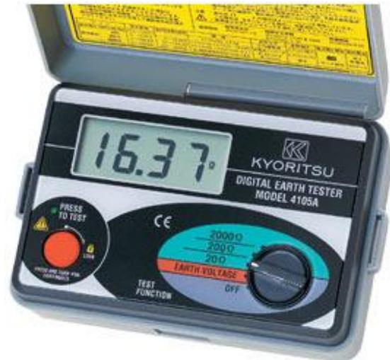
Gambar 2.4. Alat ukur earth tester
