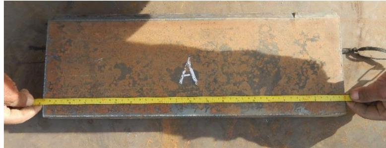
**Gambar 3. Dimensional A (40x180x500mm)**
